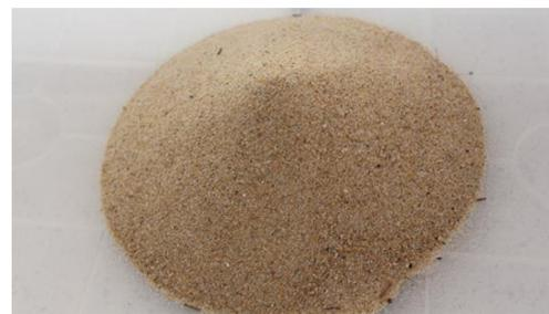
Figure 4: sample of fine aggregate
