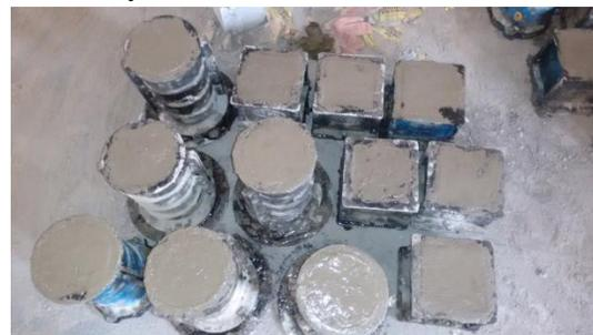
Figure 9: casted cubes and cylinders.
