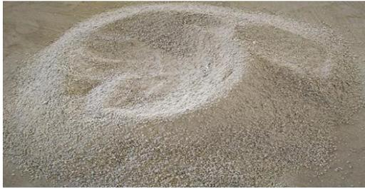
Fig 5: Sample of M-Sand
